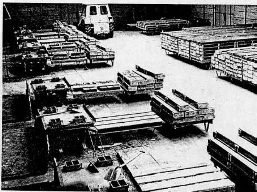
Figure 1: An historical photograph showing the start of production of concrete paving blocks in The Netherlands during the early fifties. (BKK Betonkinderdei)
