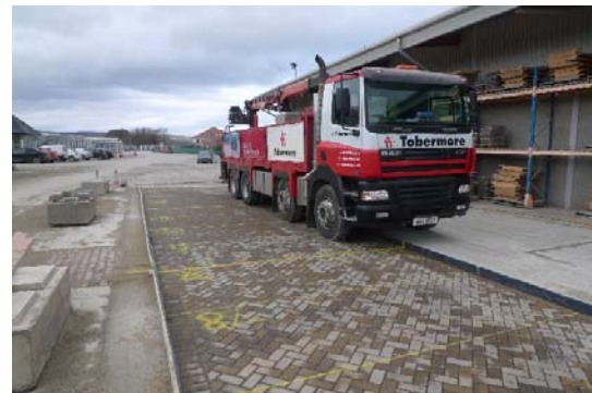
Figure 10 (left). Values of permanent deformation were measured at locations as marked on the board. Each measurement point occupied a similar position in relation to the paver laying pattern. Measurements were taken by inserting the calibrated wedge between the pavement surface and the straight edge. An initial set of readings was taken prior to trafficking and all reported readings are obtained by first subtracting the initial data set.
