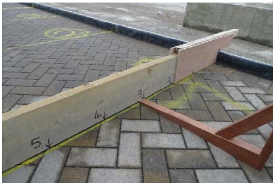
Figure 10 (left). Values of permanent deformation were measured at locations as marked on the board. Each measurement point occupied a similar position in relation to the paver laying pattern. Measurements were taken by inserting the calibrated wedge between the pavement surface and the straight edge. An initial set of readings was taken prior to trafficking and all reported readings are obtained by first subtracting the initial data set.
