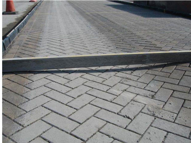
Figure 12. Typical rut in Test Item 1 after several thousand standard axles.
