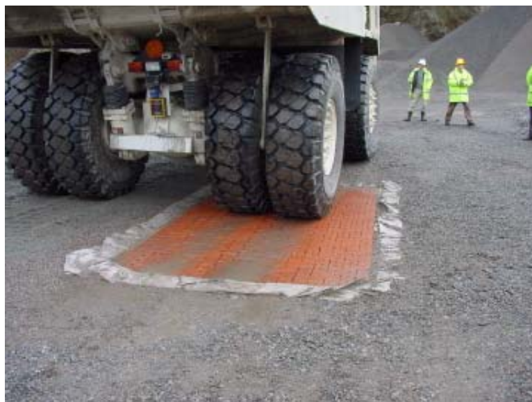
Figure 4. Testing of design section using off-road dump truck with 14t axle loads.
