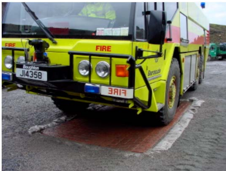
Figure 3. Testing of design section using airport's heaviest fire tender with 11.5t axle loads.
