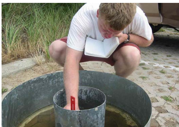
Figure 1. Double ring surface infiltration device used by Bean in 2004.
