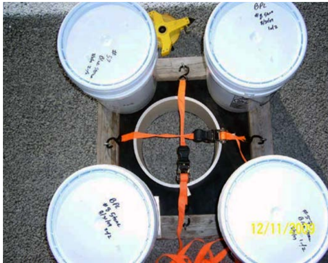
Figure 5. Modified ASTM C1701 using neoprene seal on the porous pavement (Borst 2010)
