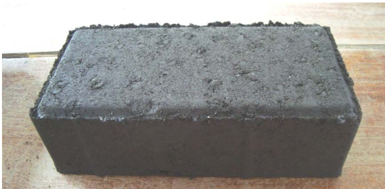
Figure 5 - Paving unit using foundry sand.
