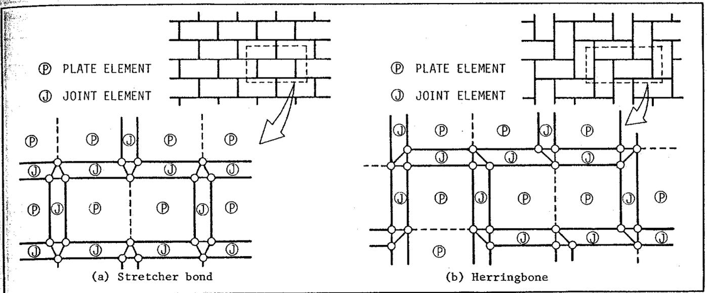
Figure 5: Idealization of interlocking block pavements.
