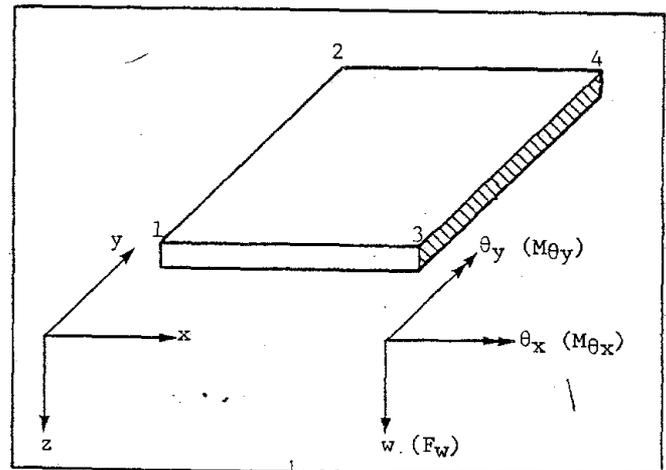
Figure 1: Rectangular plate element.
