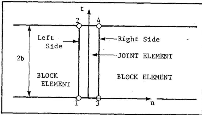
Figure 4: Joint element.
