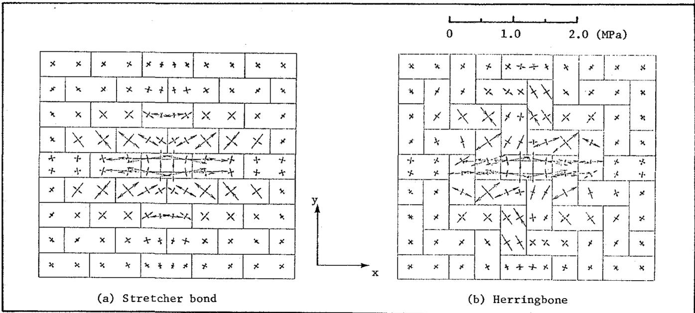
Figure 7: Distribution of principle stresses.
