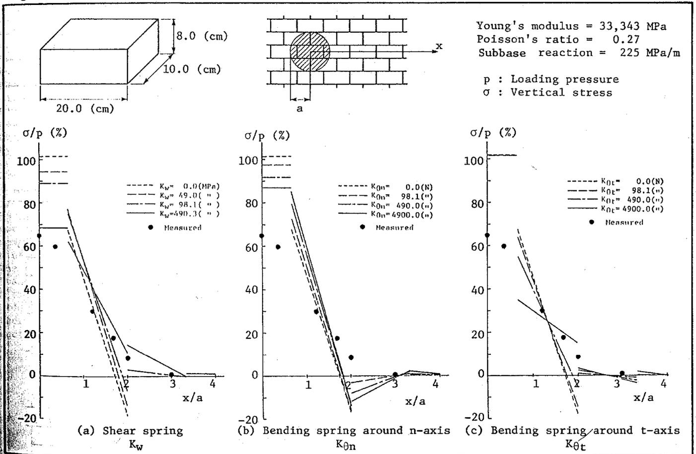
Figure 6: Distribution of vertical stress at the top of the subbase.
