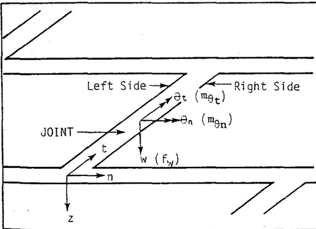
Figure 2: Coordinates and displacements of a joint.
