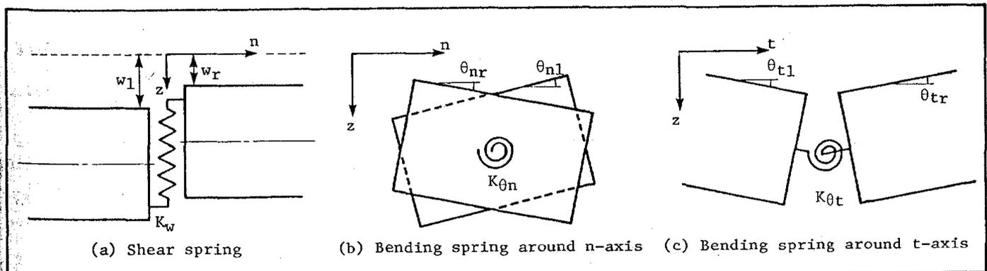
Figure 3: Modeling a joint as set of springs.
