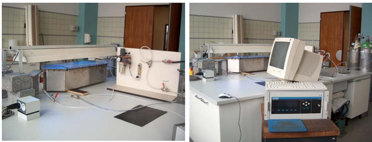
Figure 1. Set-up of the test to determine the air purifying properties with large container (3*2 rows of pavement blocks)
