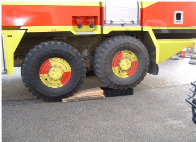
Figure 3. In order to check that Permavoid units can withstand the weight of a fire tender, a simple test was conducted to check that a unit can accept the weight of a fire tender wheel directly. This is a more onerous situation than the one which will apply in service since the load will have been dissipated by the upper pavement courses. Also, the clipping together of Permavoid units enhances their strength. The fire tender was able to remain on a single Permavoid unit for as long as required. There was minor damage to some of the Permavoid elements but the unit remained stable.
