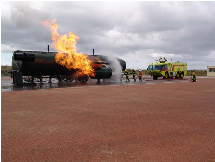
Figure 10. Fire training in operation. The brick pavers can accept the heat generated without suffering in the long or short term.
