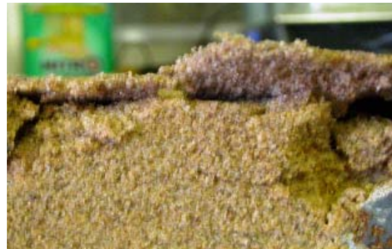
Photograph 11. Cured and uncured sand.
