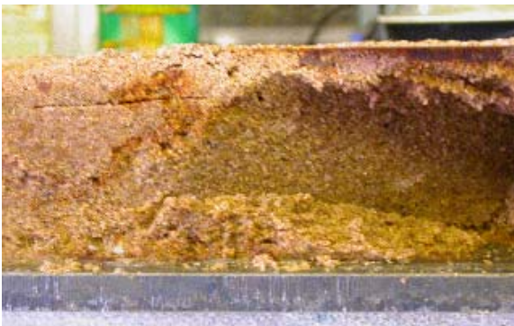
Photograph 10. Cured and uncured sand
