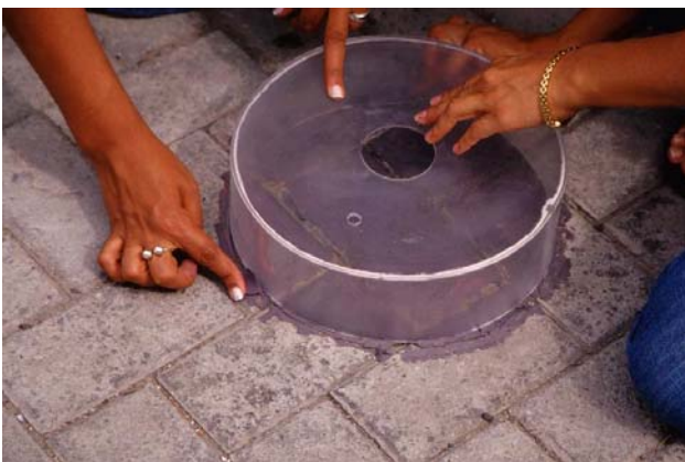
Photo 3. Sealing of the cylinder.
