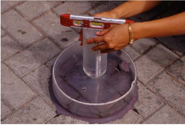
Photo 5. Leveling of the marked bottle.
